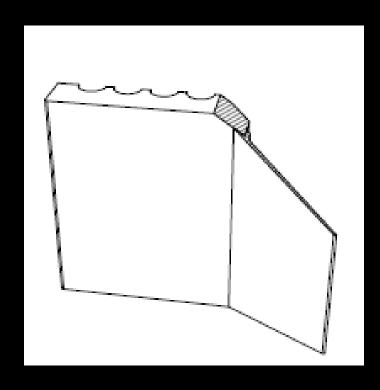
Position 2149 Uniflex™ tightly against the 2211 profile top flap head and fasten.
