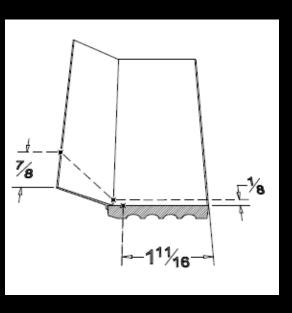
Cut 2149 Uniflex™ profile as marked. Ensure you cut through the body of the profile as indicated in the center photo. Cut piece will resemble drawing.
